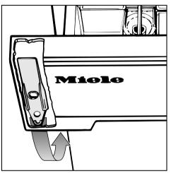
The opener for the fluff filter panel is on the side of the detergent dispenser drawer towards the rear.
